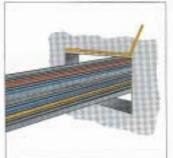
Place the lower edge of the panel first over the cables, and push slowly into the opening. Since the panel has been cut oversize, a piece of wood and a hammer will be necessary to get the panel in place. If the panel is loose in the opening, it should be discarded and replaced by a new one.
