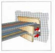
Use masking tape to keep cables and surrounding area on wall or ceiling clean.
