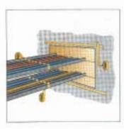
Apply KBS Coating to the edges of the panels as well as to the insides of the opening where panels will be fitted. Prior to coating application, the surface of the wall should be wetted with water.
