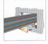
Now apply KBS Coating by spray or brush, first to panels, then to distance required by national standards. Coat wall about 2 cm over edge of opening.
