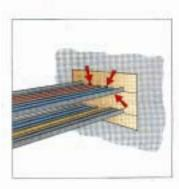
Check cut by placing panels over cables and make necessary corrections.
